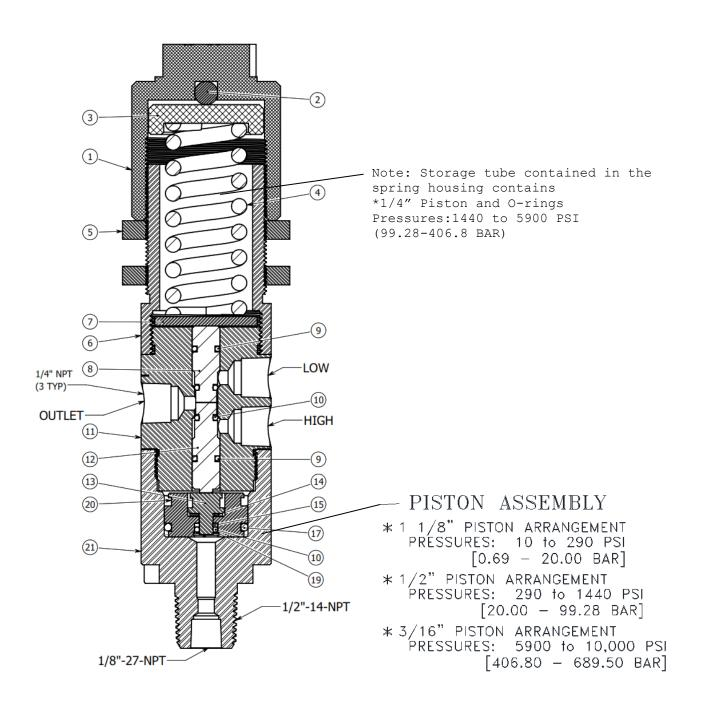
\*This piston arrangement and pressure range may be obtained through a combination of rearranging the components in the current piston assembly and utilizing components in the storage tube. The following pages contain an enlarged and detailed view with material list for each piston arrangement.
