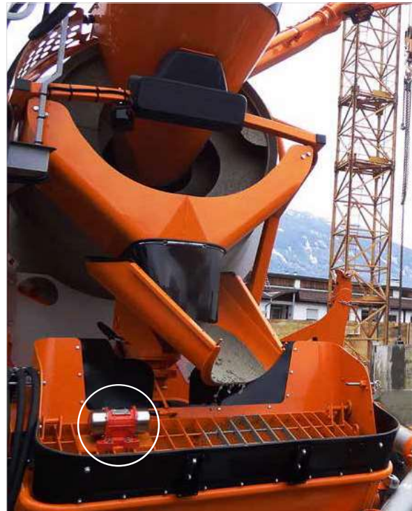
MVE-DC (electric vibrator) - Concrete pump
