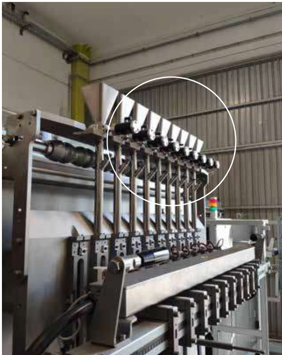
K (linear pneumatic vibrator) - Hopper emptying
