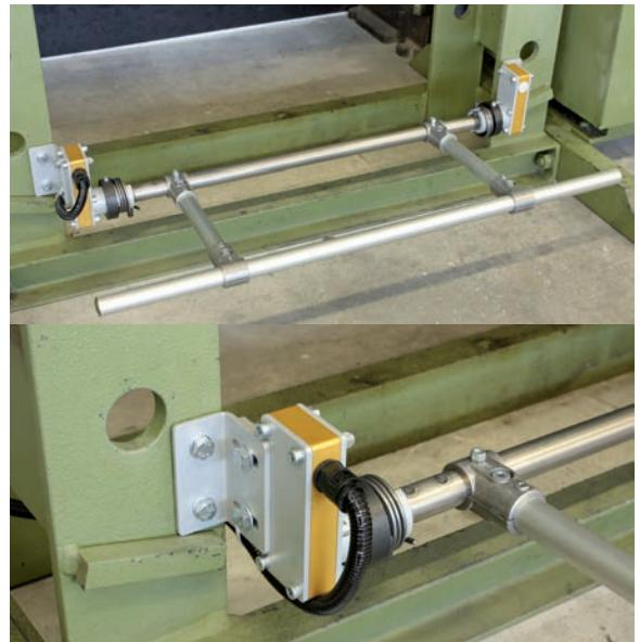
Solid and versatile device, to be used as Stop-Start - Emergency system. Operated with arms or feet. Customized on request. Available with one safety microswitch (MST-BS01/...) or a double safety microswitch (MST-BS02/...).
