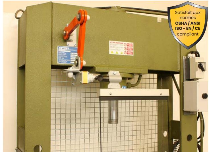
Universal articulated arms guard, with reversible opening direction. Practical and immediately adjustable. Designed for frequent changes of operation. Protects the operator from direct contact with dangerous parts frontally segregated by the shield. Frontally attachable to the machine. Equipped with wide «visibility» reversible opening shield: vertical, horizontal, left or right, with position-release knob. Equipped with a safety microswitch.
