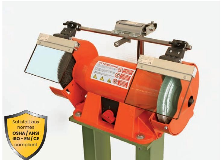
*Double-shield safety guard, supported by multi-adjustable hexagonal arms. Equipped with microswitch integrated in the support hinge.*
