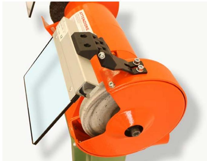
Single shield to be fixed on the grindstone cap, for protection from sparks and emery. Equipped with rubbing articulation for rapid adjustment.
