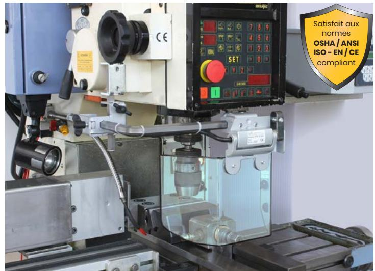
Exclusive safety guard supported by adjustable hexagonal arms. Equipped with vertical opening shield, with microswitch integrated in the rotation hinge.
