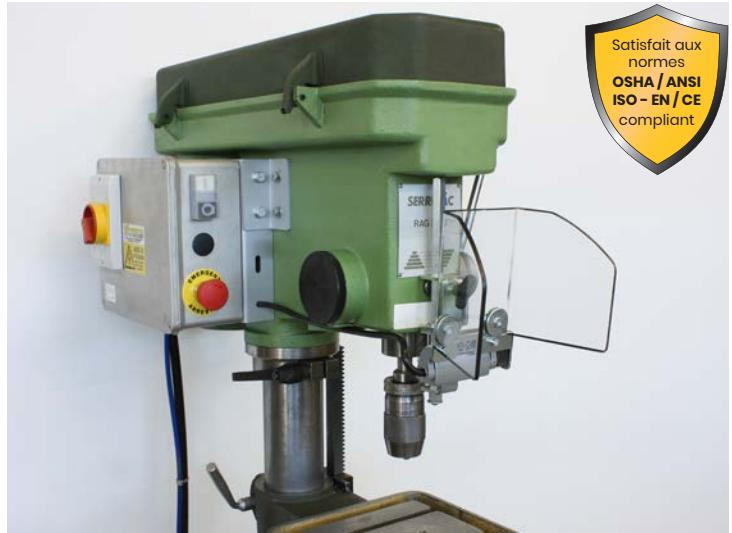
New safety shield offered with a double fixing system, supported by adjustable hexagonal arms. Equipped with a microswitch integrated in the rotation hinge.
