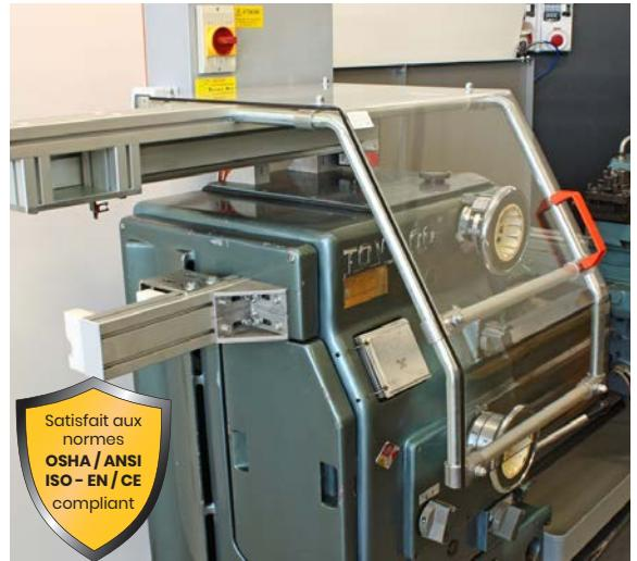
*Solid and functional safety guard. Protects the operator from direct contact with rotating components of the chuck and from the projection of shavings and lubricant-coolant. To be fixed on the machine head. It is equipped with wide «visibility» sliding shield, with various adjustments for an easy adaptation to all machines. Complete with safety microswitch.*
