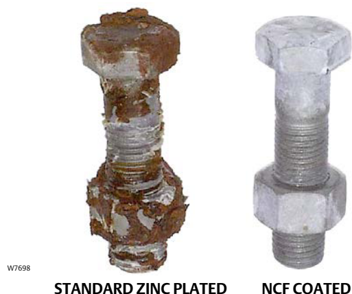
Figure 3. NCF-Coated Fasteners Exhibit Superior Performance in Accelerated Laboratory Tests
