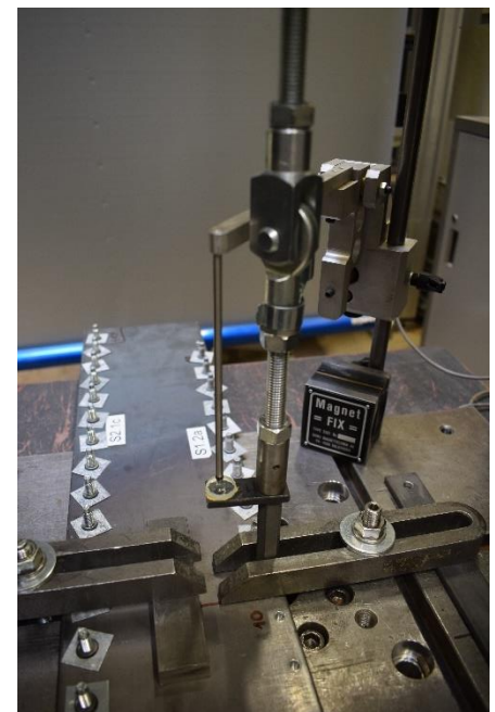
Test set up for tension tests
