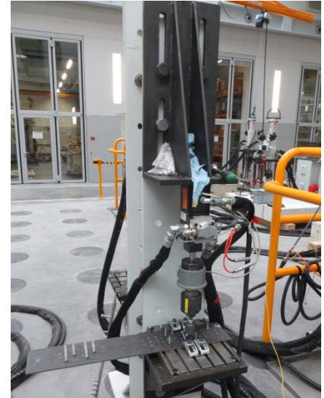
Hilti S-BT fastening system under cyclic loading
