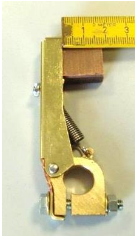
Fig. 13-11 Measuring the carbon brush
