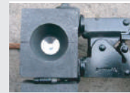
5. Place retaining disk ensuring the disk sits well at the base of the weld metal cavity
