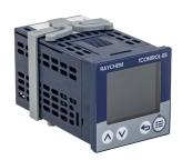
nVent RAYCHEM TCONTROL-05 is a family of single circuit electronic temperature controllers for non-hazardous areas. Most often this controller is installed in panels. Various versions of this controller are available, see datasheet for more details. Each can be used in combination with any PT100 temperature sensor or standard thermocouples. The temperature range is from -200 to 2400 °C, depending on the type of temperature sensor used.
